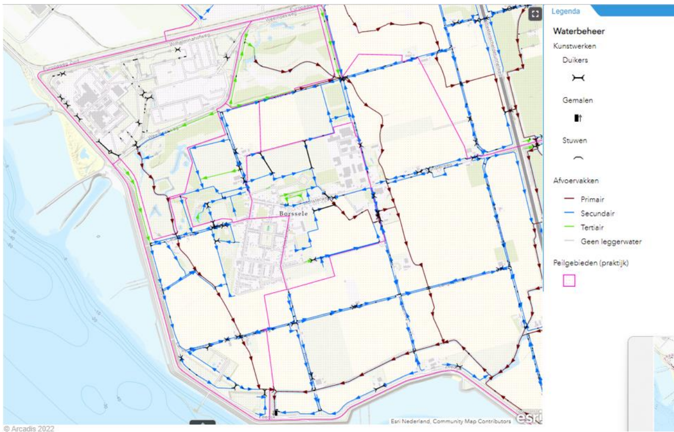
Figure 9-2 Drainage of the Borssele nuclear power plant water level area to the Borssele surface water pumping station (Waterschap Scheldestromen, 2024)
