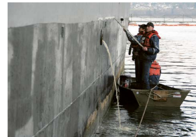
Figuur 1: Gebruik van TBT in aangroeiwerende verf op scheepswerven © Amerikaanse marine ©OSPAR Commission/courtesy of US Navy, 2017 https://oap.ospar.org/en/ospar-assessments/intermediate-assessment-2017/pressures-human-activities/contaminants/organotin-sediment/
